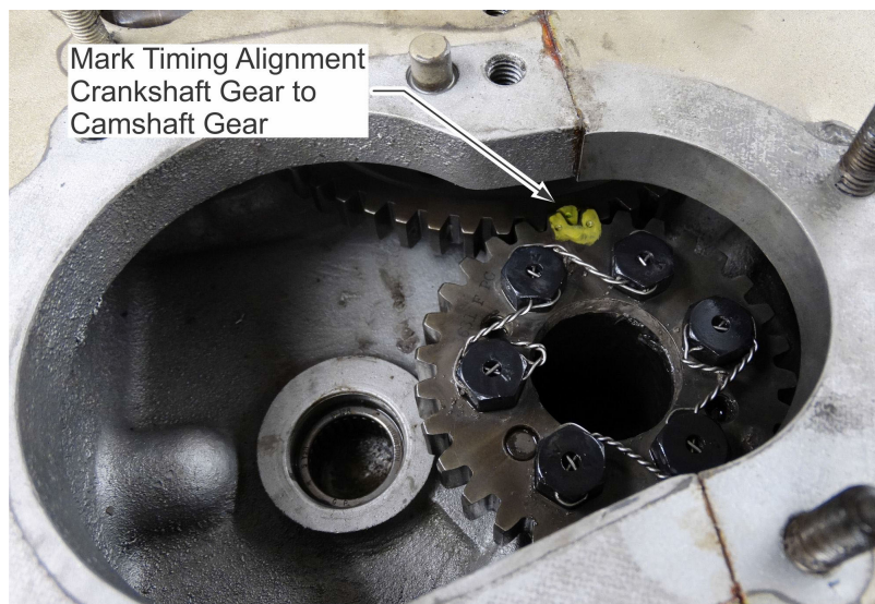
Figure 15. Camshaft Gear Timing Alignment Marked, Sandcast Crankcase
