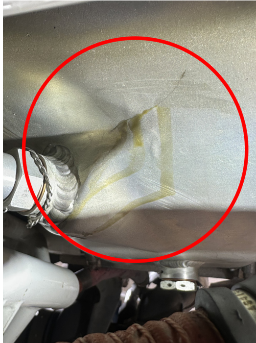
Figure 3. Affected Oil Sump Inspection Area
