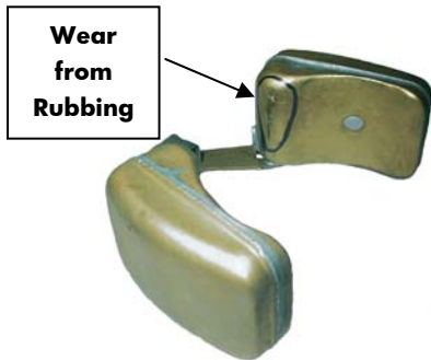
Example: Wear from Rubbing on Small MA Float Fig. 5
