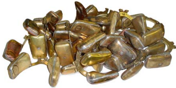
Floats with Rubbing Wear – FEB 2009 Fig. 1
