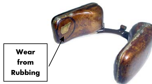
Example: Wear from Rubbing on Large MA Float Fig. 4
