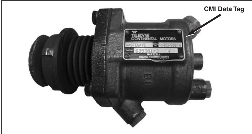
Figure 1 - Wastegate Poppet Valve Assembly (HET P/N 470892-9002 Factory Rebuilt) above (CMI P/N 635381-2 Factory New) below
