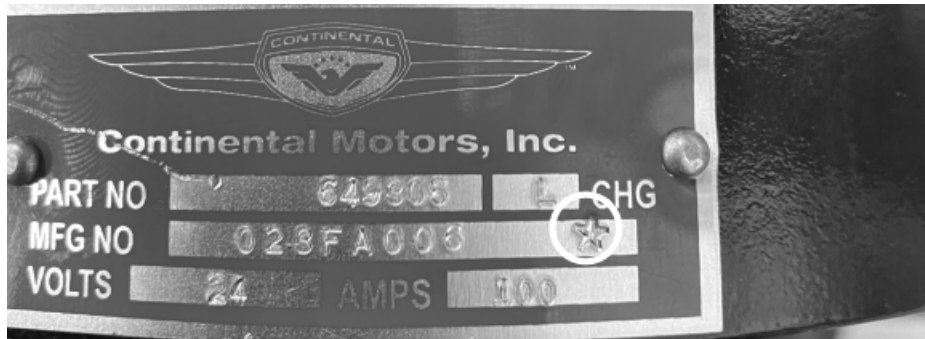
Figure 1. Star Stamp on Dataplate Indicates a Repaired Alternator
