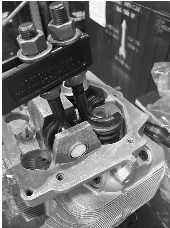
Figure 3. Compress Valve Springs with Valve Spring Compressor
